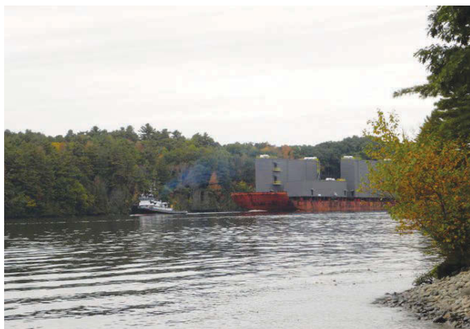
A barge loaded with prefabricated electrical buildings edges around the river bend as it makes its way to open ocean.
