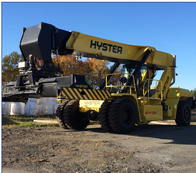
This Hyster loader will be used to expedite the loading and sealing of rail cars in preparation for the shipment of materials off site.
